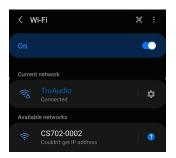
5. Once connected on your device, open a web browser and input the IP address from the front of the display to the URL bar
