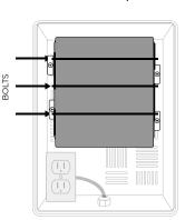
5. Loosen the horizontal bolts until they move up and down freely and insert the T100. Secure the T100 to the enclosure plate using the included velcro. Tighten the bolts to securely fasten the T100 in place.
