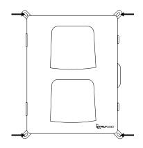
6. Use the included screws and anchors to mount the outdoor enclosure to any surface.
