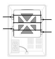
4. Install the T100/A.1x bracket using the 4 screws that were removed in step 2.
