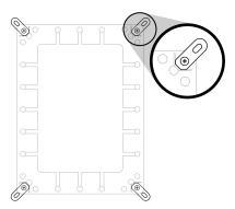
1. Install the four wall-mount brackets to the backside of the outdoor enclosure using the included screws.
