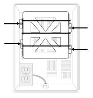
2. Remove the T100/A.1x bracket by removing the 4 screws that are securing the bracket to the enclosure plate.
